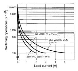
Note: A maximum current of 0.15 A can be switched at 125 VDC (cosf = 1) and a maximum current of 0.1 A can be switched if L/R is 7 ms. In both cases, a life of 100,000 operations can be expected.
